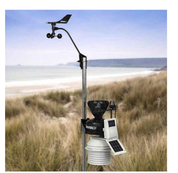
VANTAGE PRO2 PLUS (WIRELESS WITH FAN) - MODEL #6163 OR APPROVED EQUAL MANUFACTURER: DAVIS INSTRUMENTS (www.davisinstruments.com) INSTALLATION: MOUNTED ONTO IN-GROUND POLE
